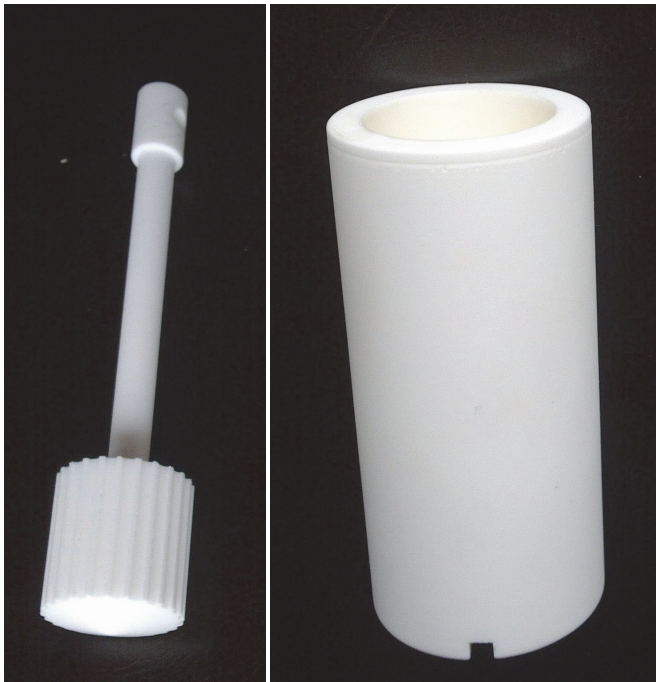
Fig. 1. Photograph of measurement tools (material - alumina) used in investigations
