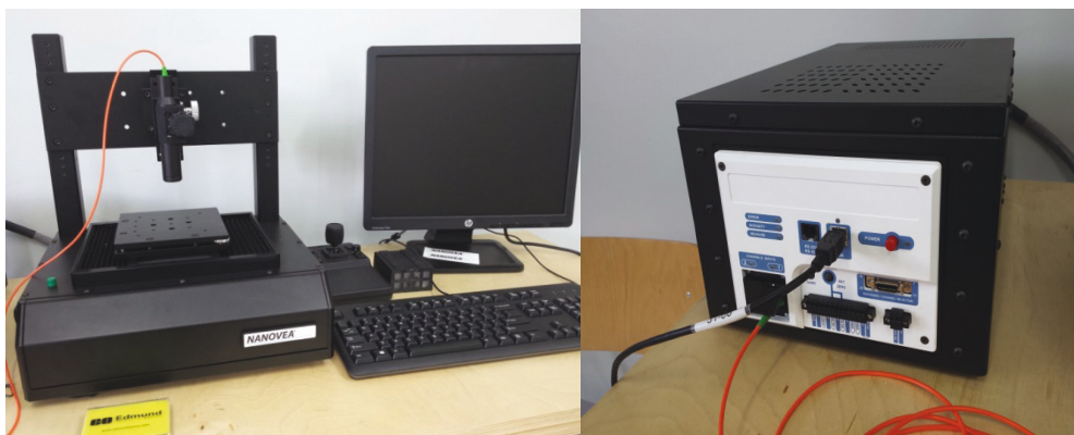
Fig. 11. Profilometer Nanovea PS50. Test stand
