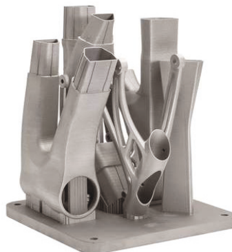
Fig. 3. Elements of the frame printed by laser sintering powders. Press Releases - Copyright Renishaw
