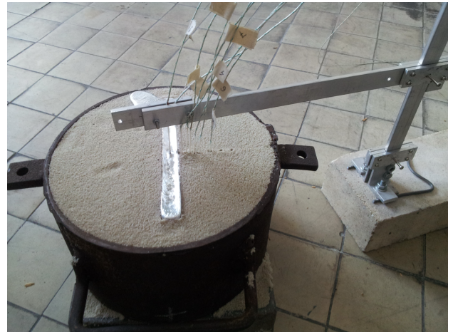
Fig. 2. The experimental mould after pouring. Visible thermocouples mounted in the mould cavity and in the mould body [9]
