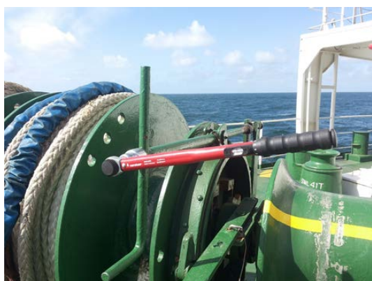
Figure 6. Torque wrench used for mooring in purpose to apply correct force on a brake related to SWL of mooring rope.
