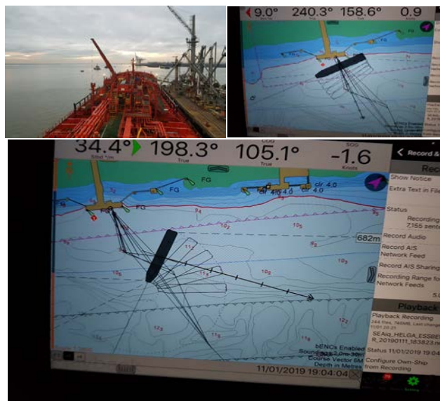
Figure 7. Example of a near miss during unmooring under strong current.
