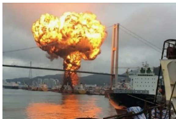
Figure 1. Chemical tanker explosion due to vigorous self-reaction of Styrene Monomer [12].
