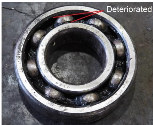
Fig. 6. Bearing failure (deterioration) [37].
