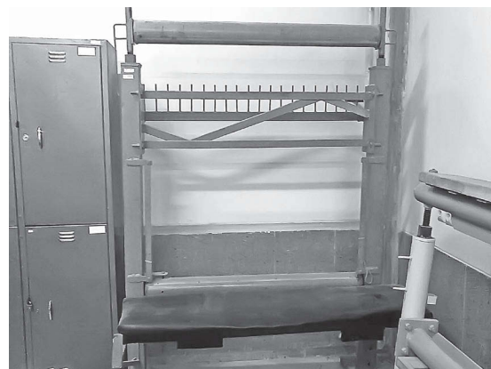
Figure 4. A rotative weaving loom built at the Carpet Department of the Islamic Art University of Tabriz, Iran.
