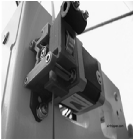
Fig. 7. The Bowden's extruder affixed to the printer's housing - as a result, the carriage with hotend is discharged, however the problems with retraction – the filament's drawing back occur (7)
