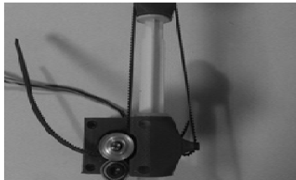
Fig. 6. The extruder for the material in the form of pulp. The force belt by means of the stepper motor is clamped around the syringe resulting in the pulp being squeezed through the extruder's nozzle (6)
