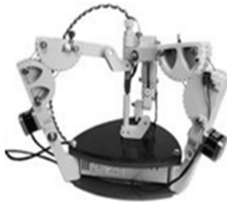
Fig. 4. The GUS - type printer – the line wrapping the arms, being clamped or released by the movement of the stepper motors, moves each of the three, independent arms (4)
