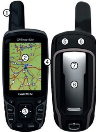
Fig. 1. Construction of the GPSMap62st receiver (GPSMap62 Series User’s Guide): 1 – internal antenna, 2 – display, 3 – keypad, 4 – POWER key, 5 – mini-USB port, 6 – MMCX connector for external GPS antenna, 7 – microSD card slot, 8 – battery
