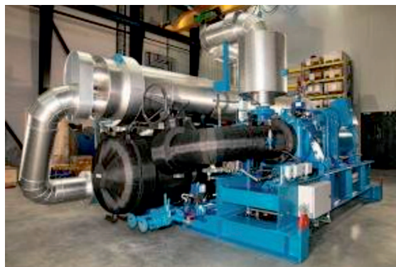
Fig. 9. Heat pump UNITOP 33C designed for boosting of geothermal well exploitation with Dogger water
