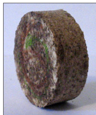
Fig. 2. Photo of a briquette obtained by the method of forming under high excess pressure, before the experiment with the determination of dynamic strength
