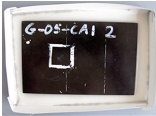
Fig. 5. Sample during immersion in epoxy resin and grinding to origin dimensions 100×150 mm
