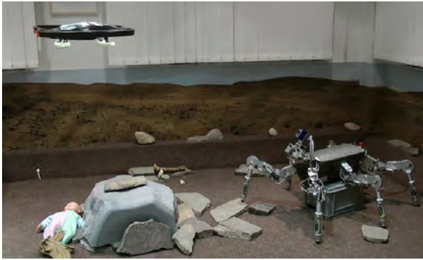
Fig. 9. LAURON is tracking the UAV which explores the area by tilting and panning its head
