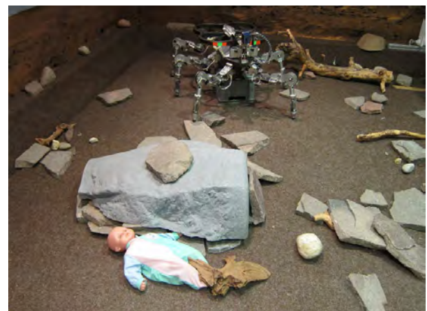
Fig. 8. Test environment that resembles the wake of a natural disaster. The environment is filled with rubble and large objects block the view of LAURON
