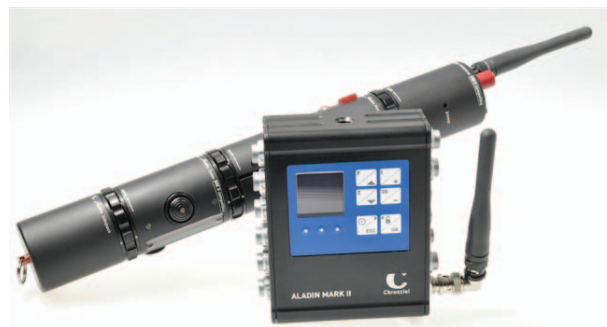
Fig. 4. Chrosziel Aladin MARK II servo motor controller and hand manipulator [8].
