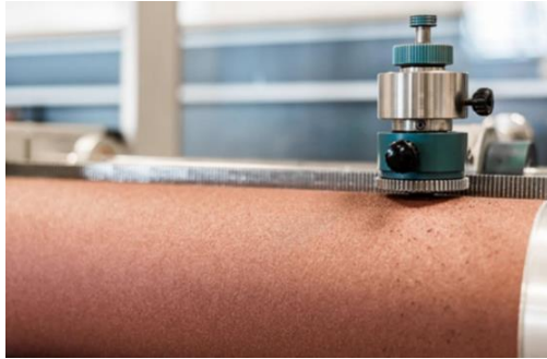
Fig. 5. Apparatus with rotating drum, including sample holder
