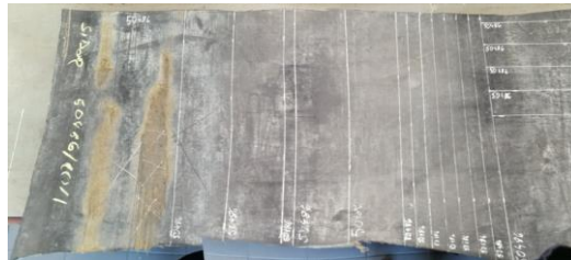
Fig. 1. Belt sample A-10, view from running cover side
