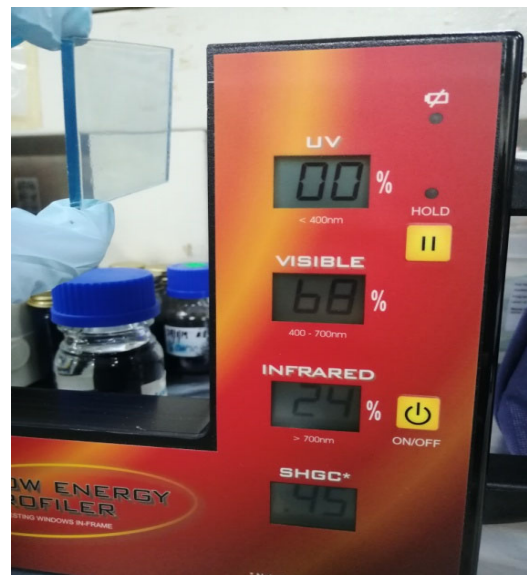
Fig. 8. WEP instrument to analyse the UV, visible light, and IR transmission on coated glass
