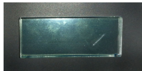
Fig. 2. Scratched or failed sample in the pencil hardness test
