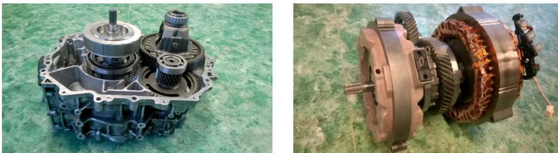
Fig. 2. Electronically controlled continuously variable transmission (eCVT)
