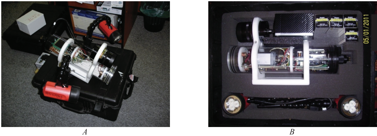
Fig. 2. Underwater photogrammetry TV camera CYKLOP: A – complete working set, B – transportive complete set
