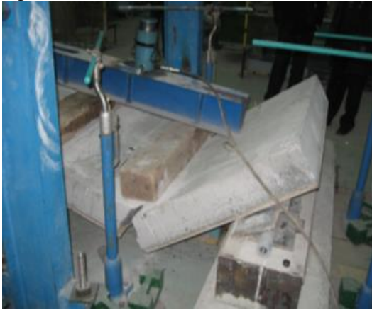
Fig. 6. The view of the slabs after destruction
