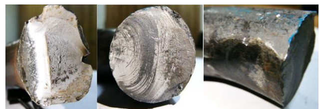
Fig. 7 Ruptured chain link
