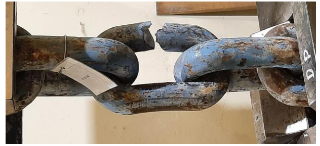
Fig. 11 The chain after fatigue testing
