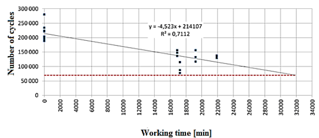
Fig. 5 Trend graph of a fatigue endurance decrease as a result of chain operation
