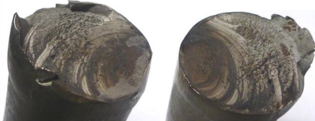
Fig. 8 Ruptured chain link
