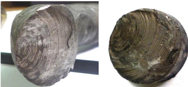
Fig. 9 Ruptured chain link
