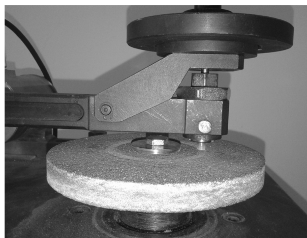
Fig. 3. A view of a friction pair on T-01M modified to test abrasive wear of metals
