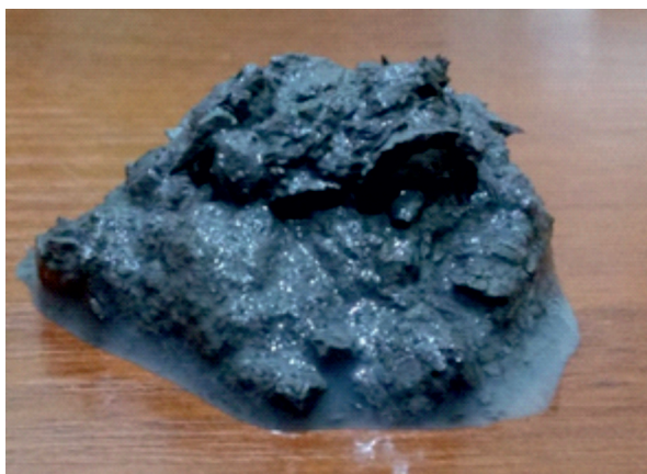
Fig. 6. Claystone from the Łaziska Beds after 10 hours in water – slake durability index r = 0.2
