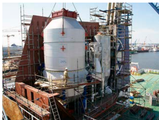
Figure 2. An assembly of scrubber installation for exhaust desulfurization (Blenkey, 2019)
