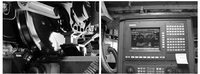
Fig. 3. One locomotive wheel under re-profiling and the measurement tool
