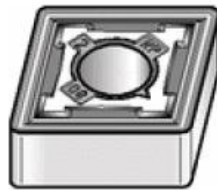
Fig. 2. Illustration of the shape of the removable cutting plate (Sasik et al., 2016)
