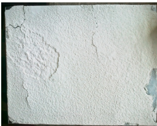
Fig. 2. Ceramic shell layer with pure Sizol030 binder
