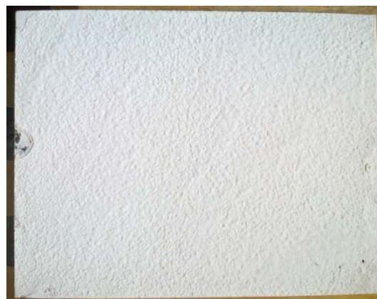
Fig. 4. Ceramic shell layer with Sizol030 binder modified with 1 mass% of C_{14}H_{10}O_4
