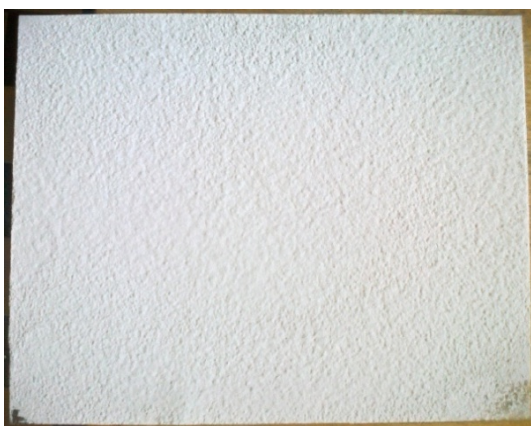
Fig. 3. Ceramic shell layer with Sizol030 binder modified with 0.5 mass% of C_{14}H_{10}O_4
