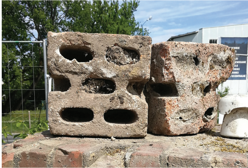
Photo 1. 'Muranów' rubble concrete breeze-block, manufactured until the 1950s; found at Kopiec Powstania Warszawskiego [Warsaw Uprising Mound]; source: the author
