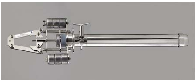
Fig. 3. Gravity corer [photo http://www.kc-denmark.dk/products/sediment-samplers/kajak-corer/kajak-corer.aspx ].
