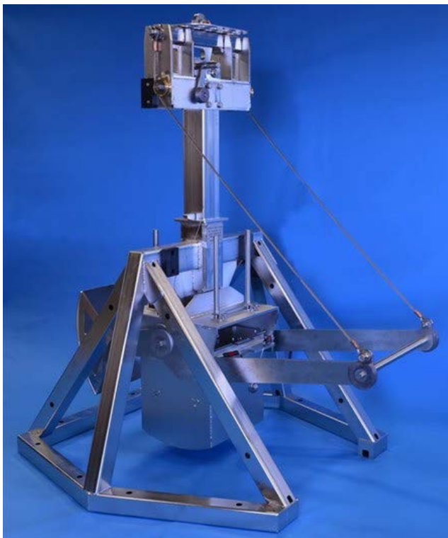
Fig. 4. Gravity corer [photo http://www.kc-denmark.dk/products/sediment-samplers/kajak-corer/kajak-corer.aspx ].
