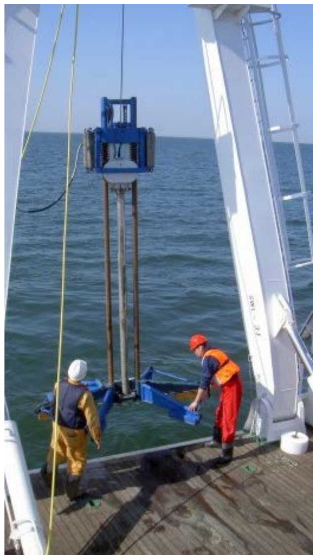
Fig. 5. Vibrocorer [photo IMG].
