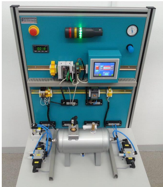
Fig. 7. Physical model of a mobile teaching stand for e-learning of PLC programming in pressure regulation
