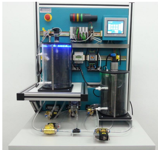
Fig. 5. A physical model of a mobile teaching stand for PLC programming e-learning in terms of liquid level control
