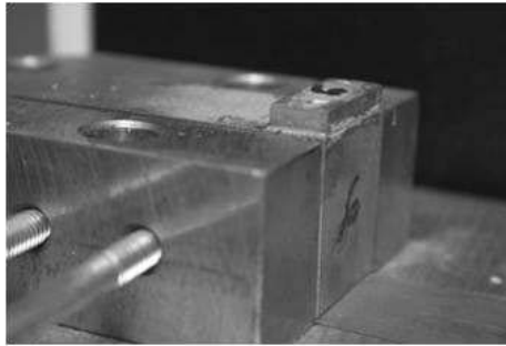
Fig. 4. Fixing of a sample in the machine hand, Galdabini Impact 25
