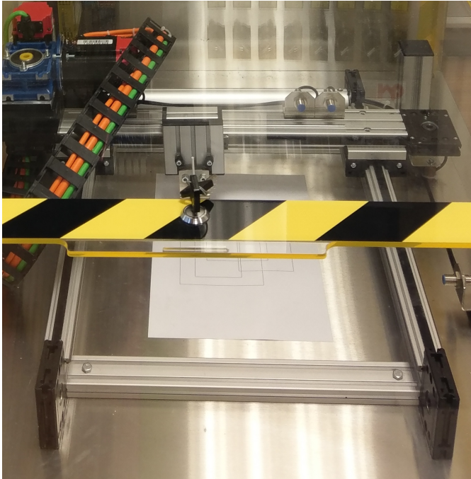
Fig. 5. 2D plotter controlled by PLC with motion controller
