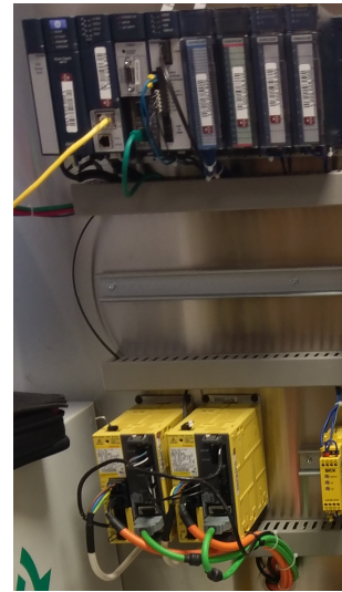
Fig. 3. Test stand – PLC with additional modules
