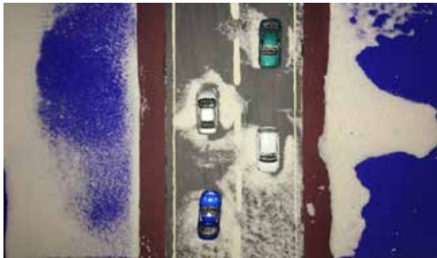
Fig. 7. Deposition of solid particles from the air flow on the model of the road with traffic-bearing surface on an embankment. One-lane traffic.
