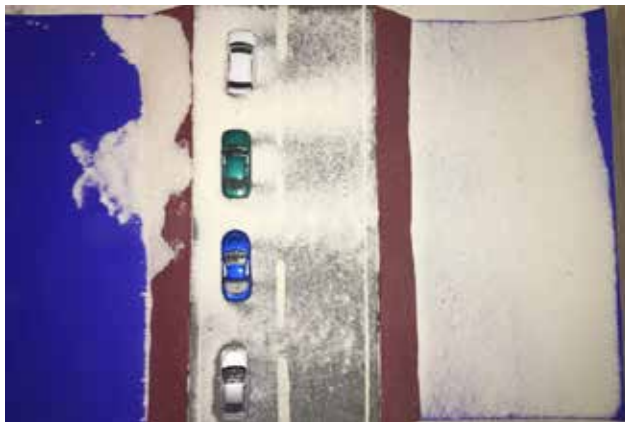
Fig. 8. Deposition of solid particles from the air flow on the model of the road with traffic-bearing surface on an embankment. Two-lane traffic.
