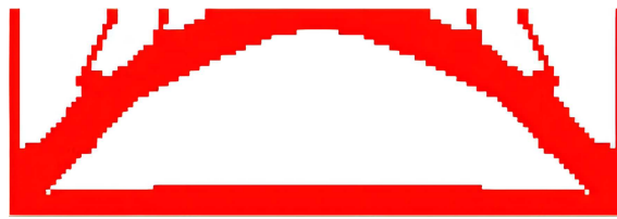
Fig. 2. Optimal topology of the short beam under a uniform load (removal rate 50%)
