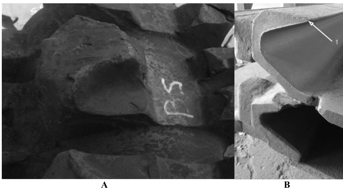
Fig. 1. Examples of tribocorrosive damage to: A – teeth of chain drums used in mining, B – sections of conveyor routes; designation: 1 – wear zone [26]
