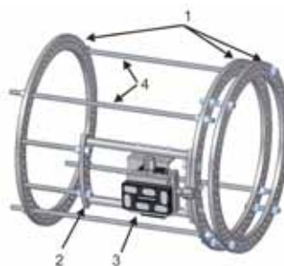
Figure 3. Ilizarov apparatus with fixing system: a) CAD model: 1 – Ilizarov rings, 2 – adaptive guides of fixing system, 3 – coupling unit of fixing system, 4 – Ilizarov ring's rods; b) picture of coupling unit of the fixing system.
