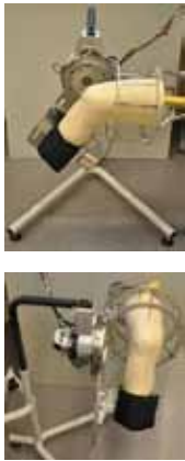
Figure 4. Rehabilitation stand consisting of rehabilitation manipulator stand, rehabilitation manipulator with mounted lower limb medical model with Ilizarov apparatus; a) lateral view, b) front view.
