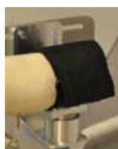
Figure 2. Shine fastening unit: a) CAD model: 1 – shine fastening with force measurement unit, 2 – shine model, 3 – fixing band, 4 – manipulator's arm, 5 – manipulator's rotational axis; b) picture of shine fastening unit with lower limb medical model.
