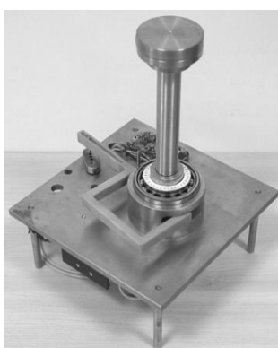
Fig. 4. View of the experimental stand with electronics and a stepper motor mounted below the base plate
