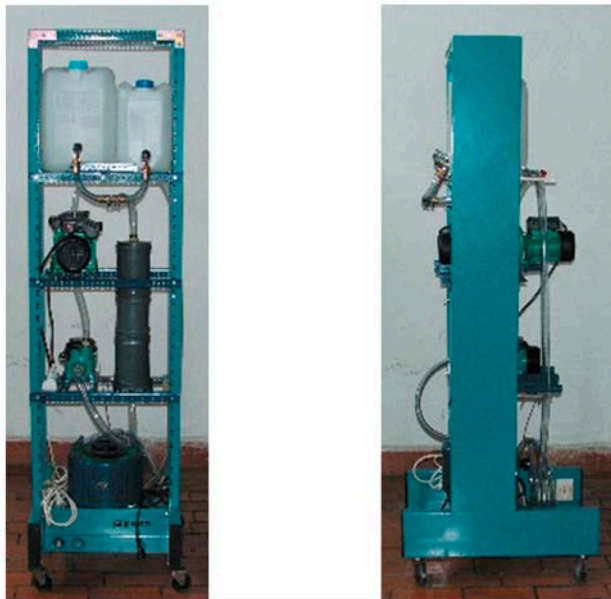
Fig. 1. Provisional facility for making the emulsion of diesel oil + water
