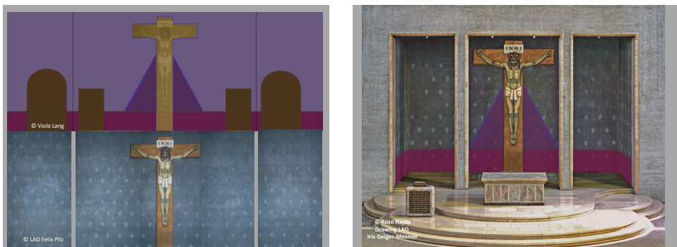
Fig. 8 Comparing a schematic design with the photogrammetry of the present situation, showing that the doors and the niches were bricked up, plastered and overpainted (Schematic design: Viola Lang, Ulm; photogrammetry: LAD BW, FG Baudokumentation)
