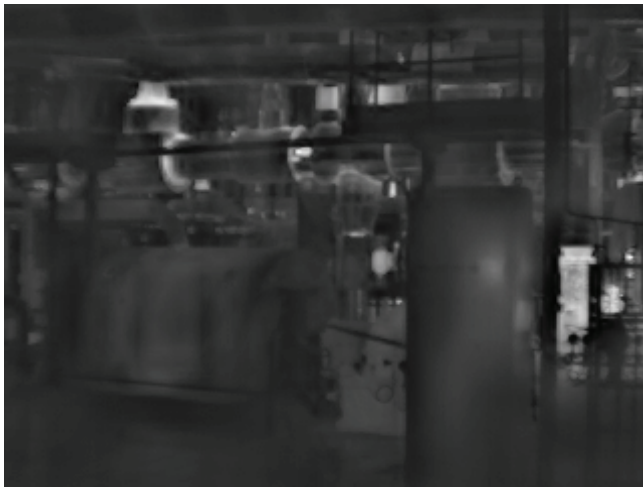
Fig. 6. Exemplary aggregated image using DWTF-GDF scheme with wavelet Sym4 and fusion rule Max, weighting function parameter k=-1.01 , number of images in considered LSSI and HSSI sets N=128 (PSNR = 15.30)
