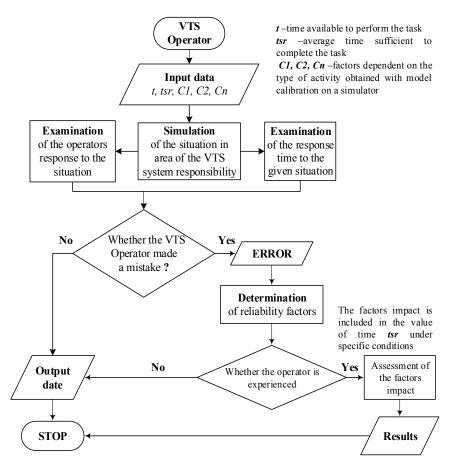
Figure 5. Block diagram of the simulation method
