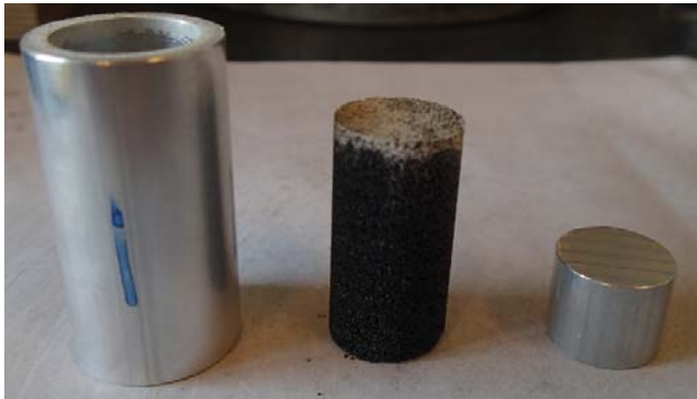
Fig. 1. Pictures of cylindrical mould (left), coated sand sample (centre) and aluminium spacer used for compaction (right)
