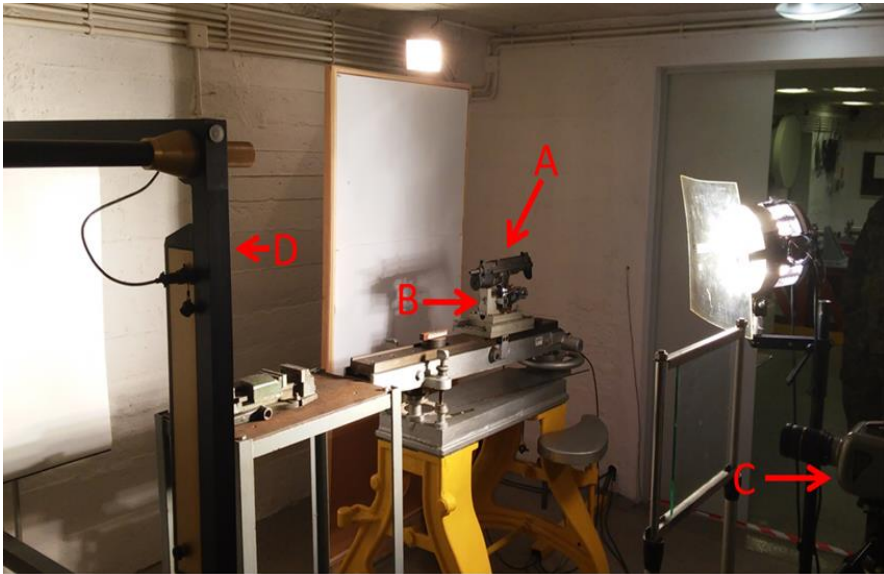
Fig. 1. Measurement set – up (A – investigated pistol, B – ballistic mount, C – high speed camera, D – precision light screen B-470)
