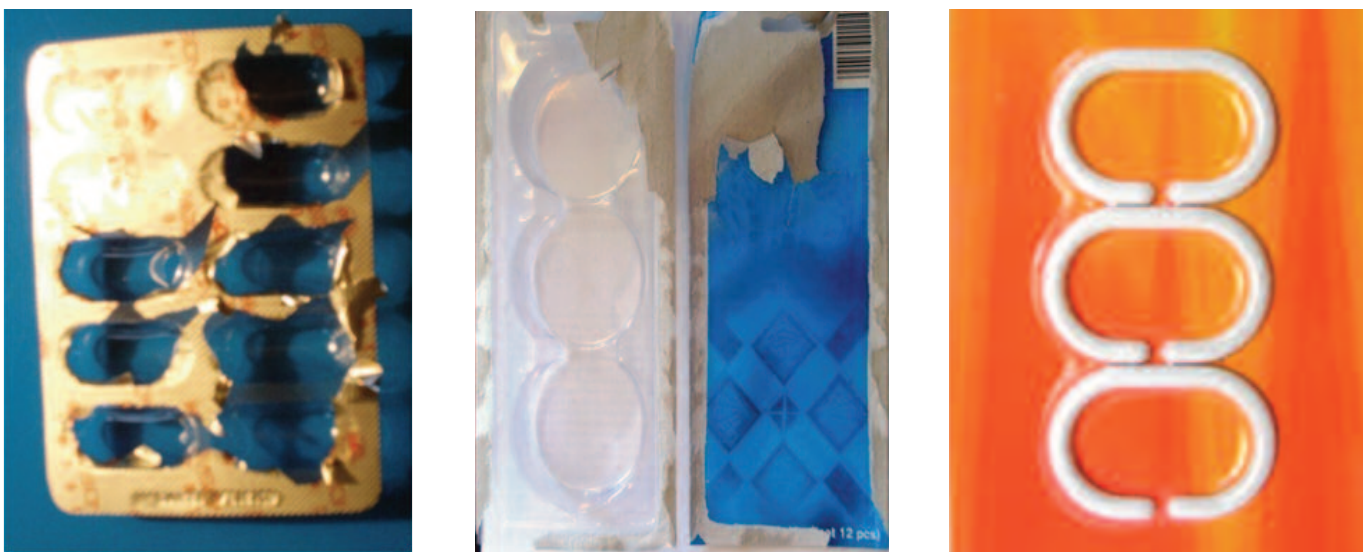
PIC. 4. THE EXAMPLES OF COMPOSITE PACKAGING OF BLISTER AND SKIN TYPE WHERE THE LAYERS MADE OF DIFFERENT MATERIALS CANNOT BE SEPARATED
