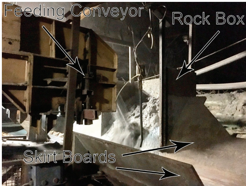
Fig. 1. A transfer station with rock box in underground mine
