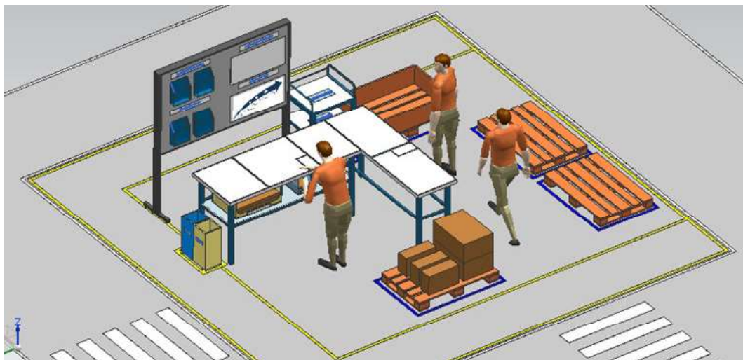
Fig. 3. Visualization of the projected assembly workstation in NX10 [6]
