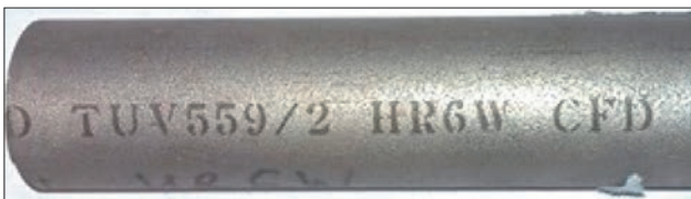
Fig. 1. Section of an HR6W (23Cr-45Ni-6W-Nb-Ti-B) alloy superheater coil
