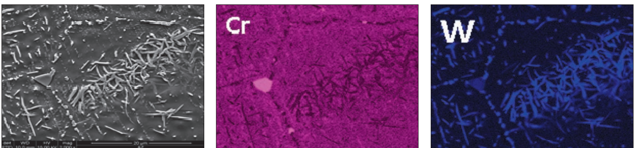
Fig. 10. Distribution of chromium and tungsten concentration in the microstructure of the HR6W alloy after ageing at 750°C for 10,000 hours. SEM observation (map of precipitates)
