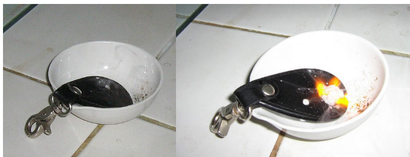
Figure 2. Ignition of leather exposed to direct contact with 98% hydrogen peroxide
