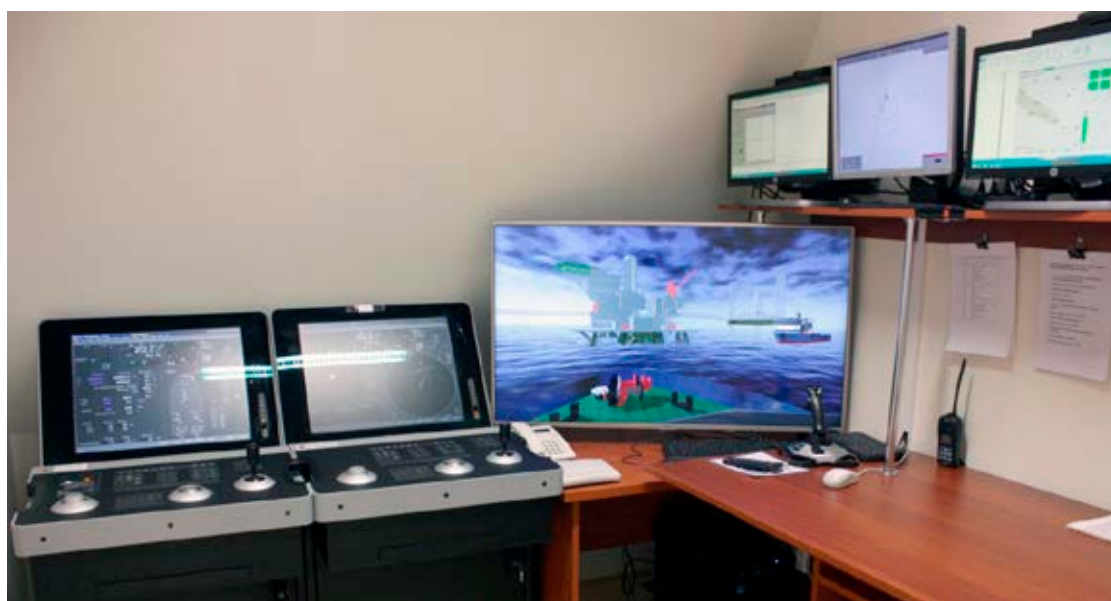
Figure 5. DP simulation system with thruster allocation and vision prepared at MUS. From left to right: two operator control stations, vision display, electronic position fixing systems screens and electronic site chart screen
