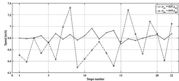
Fig. 7. Speed behavior of the electrical bus in the route [own study]
