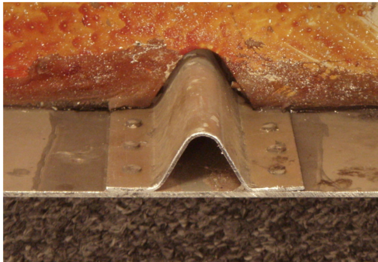
Fig. 5. Longeron (internal view)
