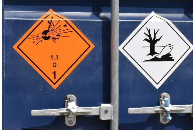
Fig. 4. Labels shall be in the form of a square set at an angle of 45°
