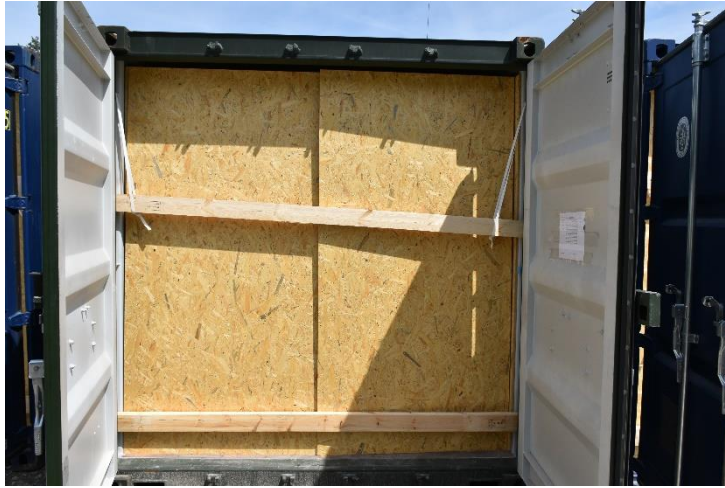
Fig.7. The cargo is secured against movement towards the door.
